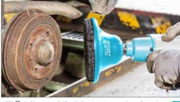
$\bullet$  With  ${\ensuremath{\,\boxtimes\,}} \ensuremath{\,^{1\!\!\!/}}$  inside square collet for attachment e.g. to pneumatic, cordless and corded impact wrenches
